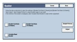
8 Select the state of the fold and staple position of the printout, and enter the 2-sheet stack misalignment amount you measured in step 6 in [Values A & B Before Adjustment].
