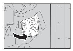
**3** With grasping the orange lever, pull out the staple cartridge.
