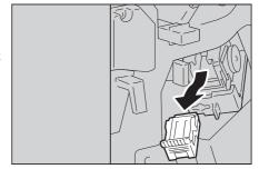
• When the C3 Finisher Staple Unit 65 Sheets is installed, pull down the orange lever, and pull out the staple cartridge.
